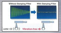
of the axis stopping. The number of filters has been increased to four from the conventional two filters (two for simultaneous use). The adaptive frequency has also been significantly expanded from 1 to 200Hz.
