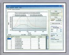
A5L drive equipped with a simplified machine simulation function, which uses frequency response data acquired from the actual machine. It also features machine simulation function for performing simulated operation.
