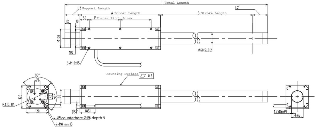
Note: Cable length 300mm. The bending radius of the motor cable should be 36.6mm (wire diameter 8.9 \* 6) as suggested by the wire manufacturer. This radius should be maintained. Use supplied connector to attach the proper high-flex cable as required by your application.
